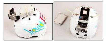
There is in the front a waterproofed <u>GoPrp</u> camera. And in the back the <u>FollowMe</u>-Transmitter with 9V batterie supply and a WI232 transmitter.
