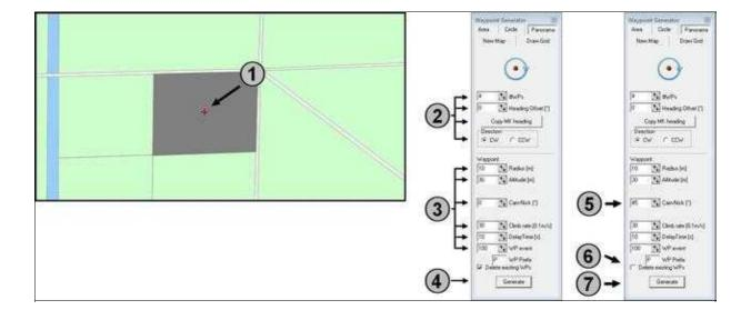
After a "click" on "Create" (4) the first WayPoints (No. 1-4) will be entered into the Editor. Then, after changing the tilt (5) and taking off the checkmark in "Delete existing WPS" (6) and been "clicked" again on "Create" (7) the new WayPoints (No. 5-8) with the new tilt appears in the editor under the already existing ones:
