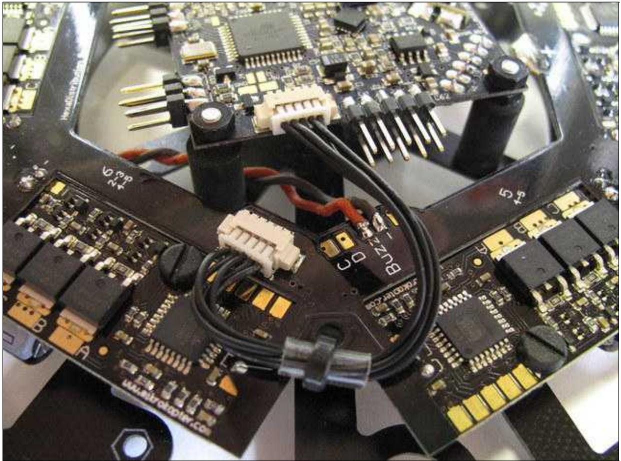
⚠ The printed arrow on the [FlightCtrl](#) must show to the on the rigger No.1 (red rigger) !
