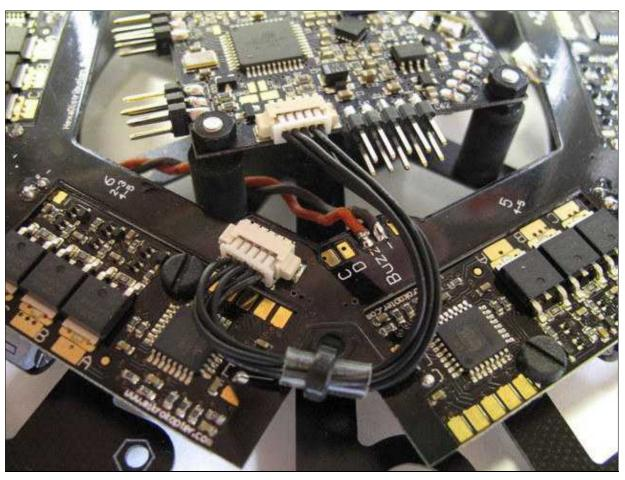
⚠ The printed arrow on the FlightCtrl must show to the on the rigger No.1 (red rigger)!
