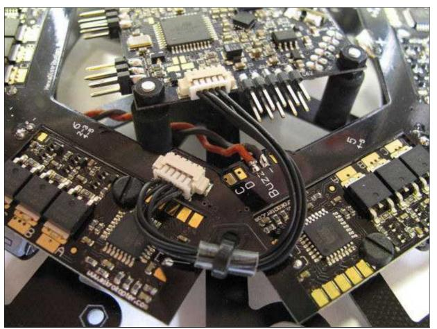
A The printed arrow on the FlightCtrl must show to the on the rigger No.1 (red rigger) !
