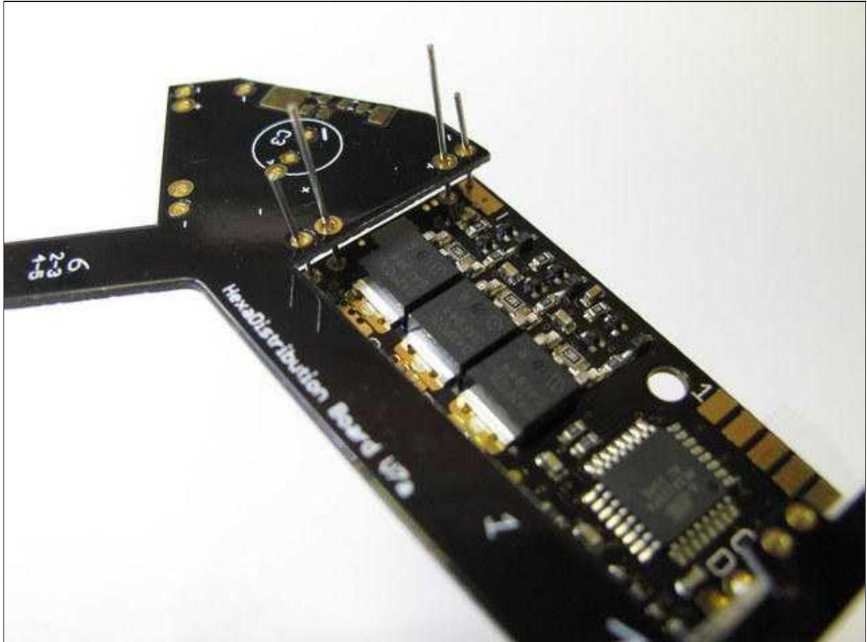
When soldering the capacitors and the I2C bus, take care that the BL-Ctrl2.0 applied directly to the power distributor.
