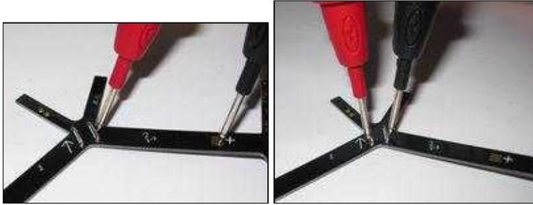
To measure with a multimeter: All points must have a high impedance to each other --> higher than 100kOhm respectively the multimeter doesn't show anything. (The BL-Ctrl's are not soldered in at this point)
