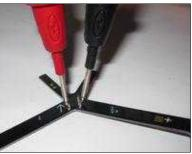
To measure with a multimeter: All points must have a high impedance to each other --> higher than 100kOhm respectively the multimeter doesn't show anything. (The BL-Ctrl's are not soldered in at this point)
