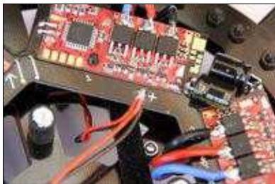
To those +/- pads of the distribution-board for the power supply of the FC the cable for the LED-stripe of the front rigger will be soldered down there and of course right in polarity.
