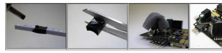
The sensor can now be pushed down slightly on the board. The shrink tube is fitting now tight to the foam above the air pressure sensor. This attachment is sufficient and must not be shrunk any further.
