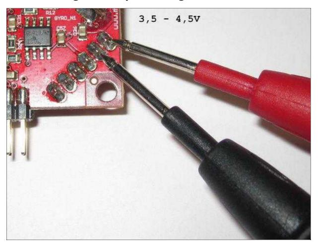
With a multimeter you can check the output voltage of the sensor slightly.
