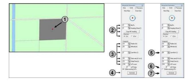
After a "click" on "Generate" (4) the first WayPoints (No. 1-4) will be entered into the Editor. Then, after changing the tilt (5) and removing the check mark in "Delete existing WPS" (6) and "clicking" again on "Generate" (7) the new WayPoints (No. 5-8) with the new tilt appears in the editor under the already existing ones:
