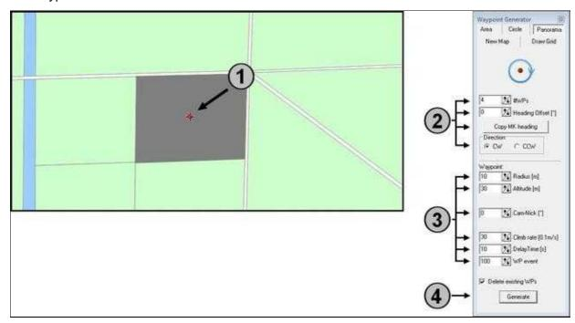
After a "click" on the button **"Generate"** the WayPoints with the settings will be entered automatically into the **WayPoint-Editor**.
