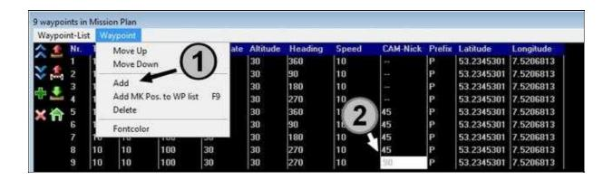
Now the WayPoints can be transferred to the Kopter and been flown. How that works is described under <u>"The WayPoint-Flight"</u>.
