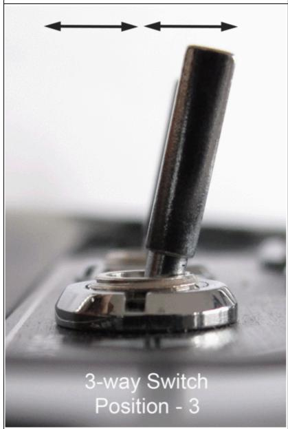
Position 3 = An (254) Trigger the camera manually
