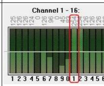
To use the Automatic during a Way point flight we have to change the settings for this channel on the transmitter. If you use e.g. a Graupner HoTT transmitter we find this setting under *Servo adjustment*: (in this example we use channel 11 to trigger the camera)
