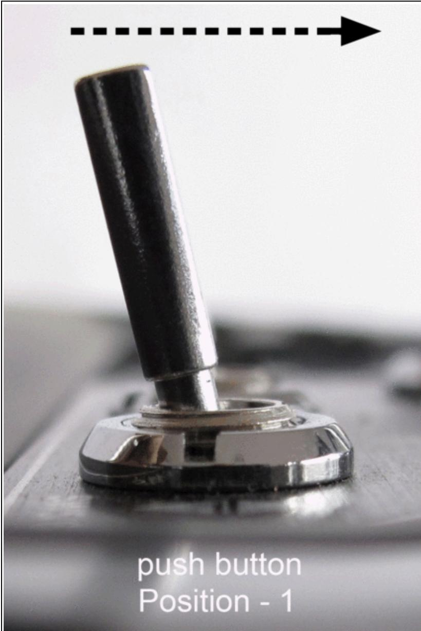
without activation = Automatic (126) Camera will not trigger. (Automatic triggering during a WP-Event)
