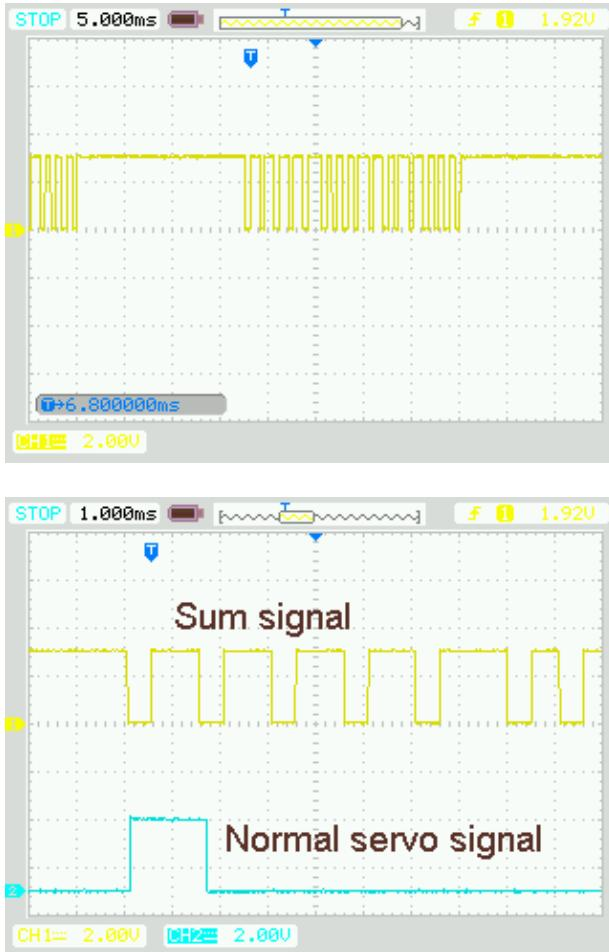
The [FlightControl](#) operates with an inverted signal also. No change in the settings required.
