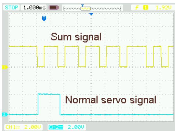
The [FlightControl](#) operates with an inverted signal also. No change in the settings required.
