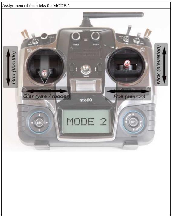
Description of the stick assignment for MODE 2 Calibration of the ACC Function (One time => necessary. The Kopter Nick (elevation) must stand Gas (throttle) straight.) Throttle up Description / Yaw right of the stick assignment / Nick middle / => Roll middle Gier (yaw / rudder) Roll (aileron) mx-20
