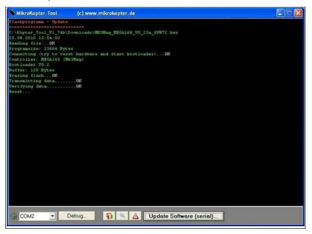
After the update an automatic reset is performed and the unit restarts. In the Terminal Window you can see now the initialization of the module.
