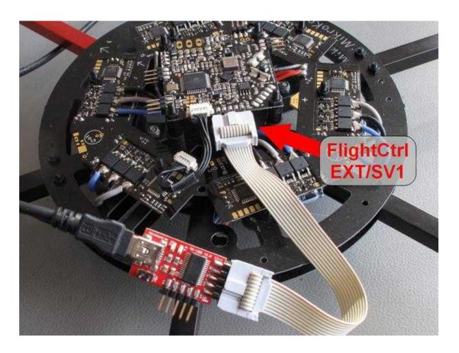
However, if the MK-Tower is used at the MikroKopter (FlightCtrl, NaviCtrl, MK3Mag, MK-GPS), the FlightCtrl and the NaviCtrl are connected over a 6-pin and one 10-pin cable.
