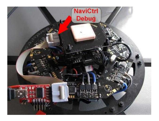
**The jumper on the MK-USB is still open.** To power the <u>MikroKopter</u>, please use the lipo or a power supply. A regulated power supply is particularly recommended for the first start of the <u>MikroKopter</u> to avoid damage to the Kopter
