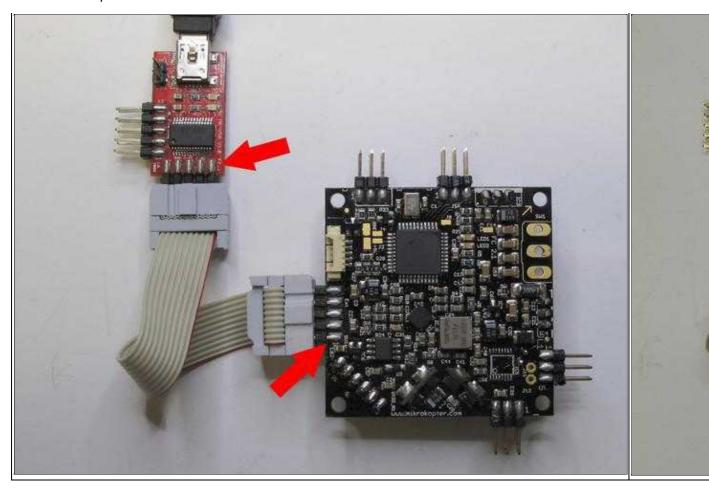
If the boards, as shown in the pictures, are individually connected, the voltage supply is supported by the MK-USB.
