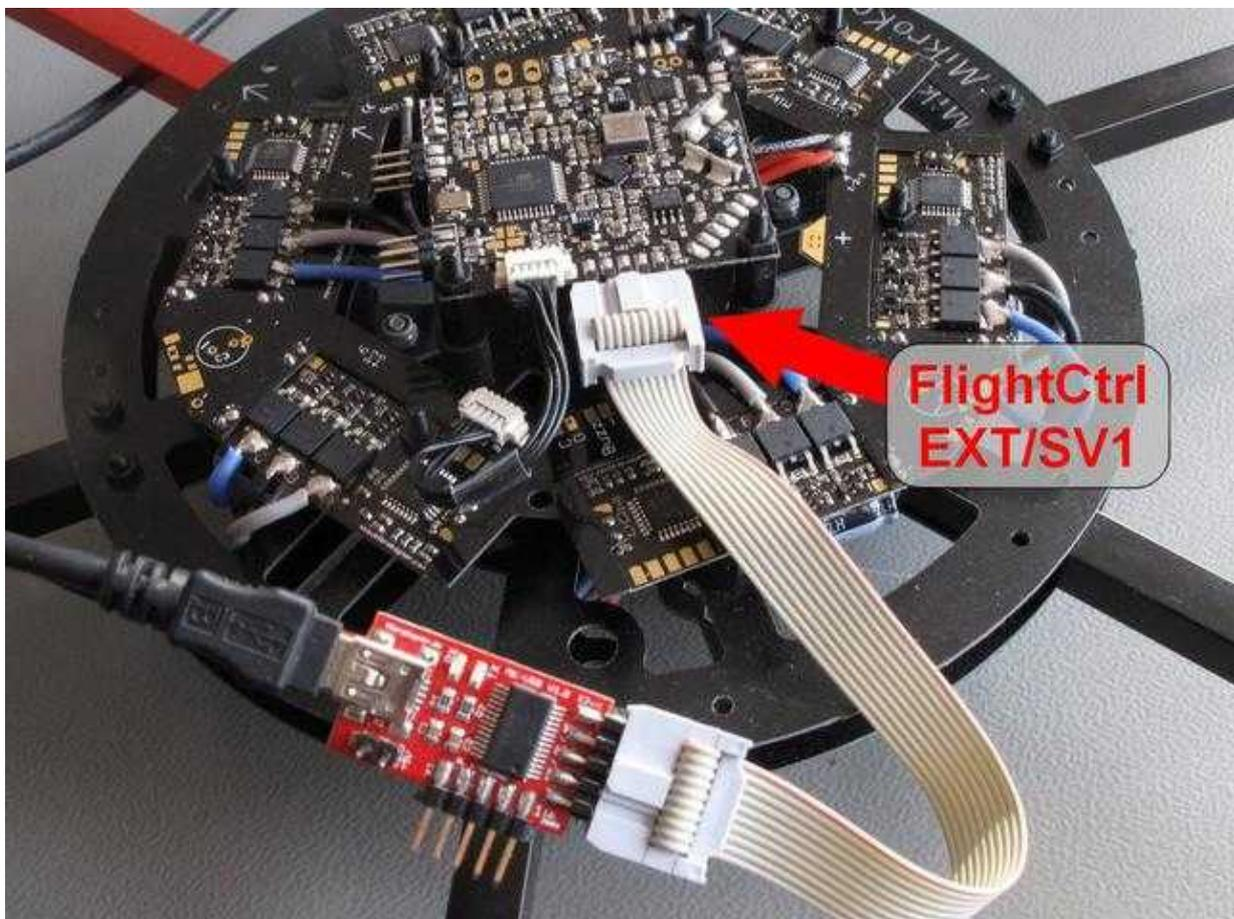
However, if the [MK-Tower](#) is used at the [MikroKopter](#) (FlightCtrl, NaviCtrl, MK3Mag, MK-GPS), the FlightCtrl and the NaviCtrl are connected over a 6-pin and one 10-pin cable.
