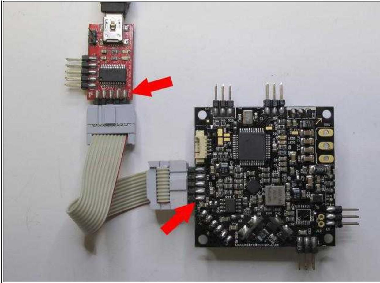
**i** If the boards, as shown in the pictures, are individually connected, the voltage supply is supported by the MK-USB.
