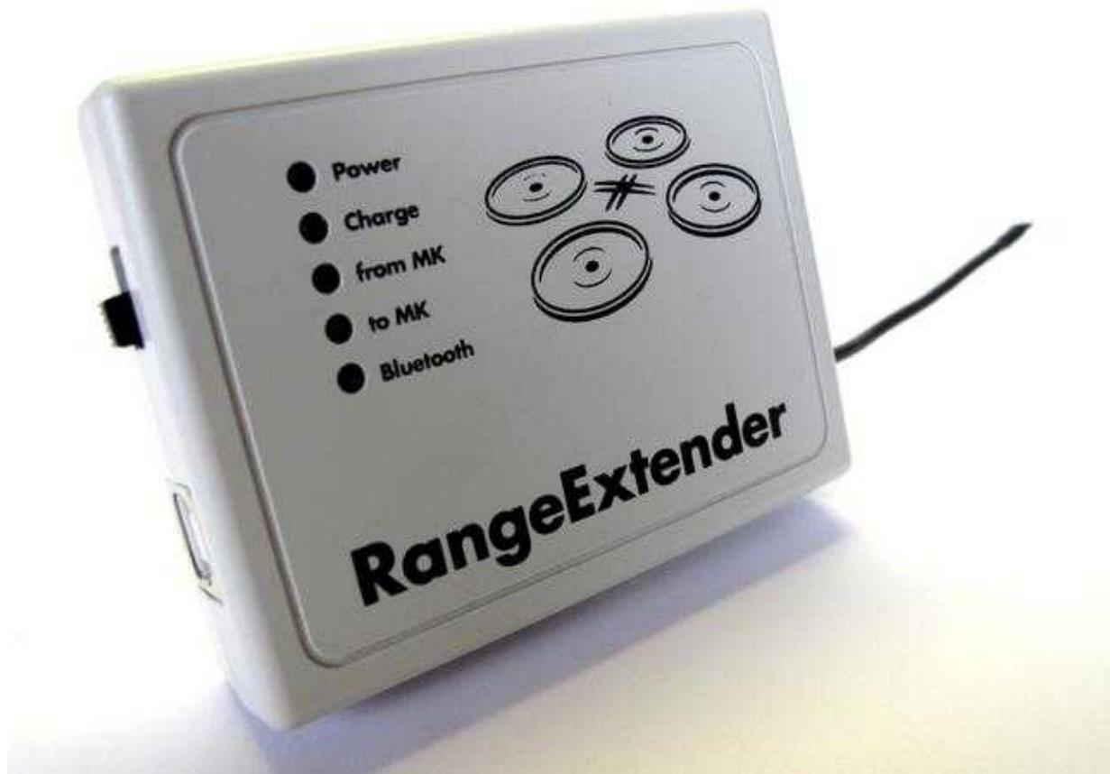
With the RangeExtender, a wireless connection can be established to the MikroKopter over a large range (>1000mtr).
