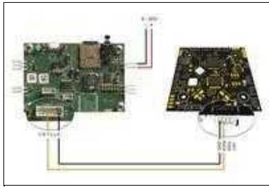
The "RTK-GPS-receiver" (in this example a *Septentrio AsteRx-m2* UAS receiver) is connected with **RxD2** and **GND** at the **UART2**-port.
