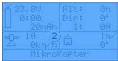
The RTK-GPS (if set correctly) is automatically detected by the MikroKopter.
