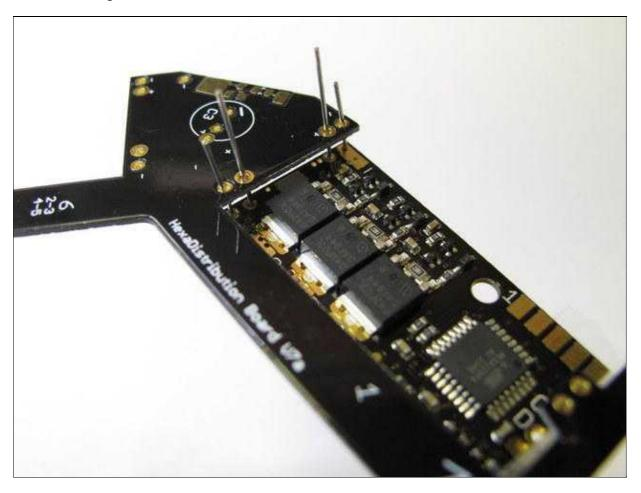
When soldering the capacitors and the I2C bus, take care that the BL-Ctrl2.0 applied directly to the power distributor.
