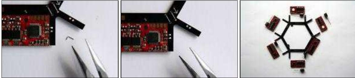
The silver wire will be stuck in the holes of the distribution-board and bent over. After that the ends of the wires will be soldered to the "C" and "D" connection pads of the BL-Ctrls.
