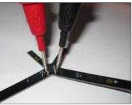
To measure with a multimeter: All points must have a high impedance to each other --> higher than 100kOhm respectively the multimeter doesn't show anything. (The BL-Ctrl's are not soldered in at this point)
