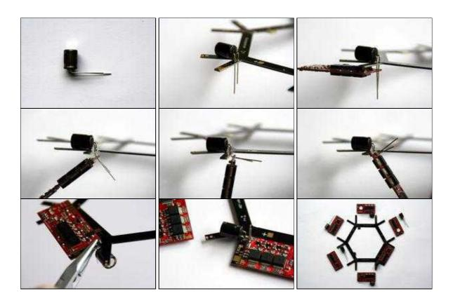
A You need to solder all Elkos carefully and with alot of heat otherwise you'll get pretty quick a cold solder-joint. The distribution-board is covered with 70μm copper so that more heat can be discharged to the sides.
