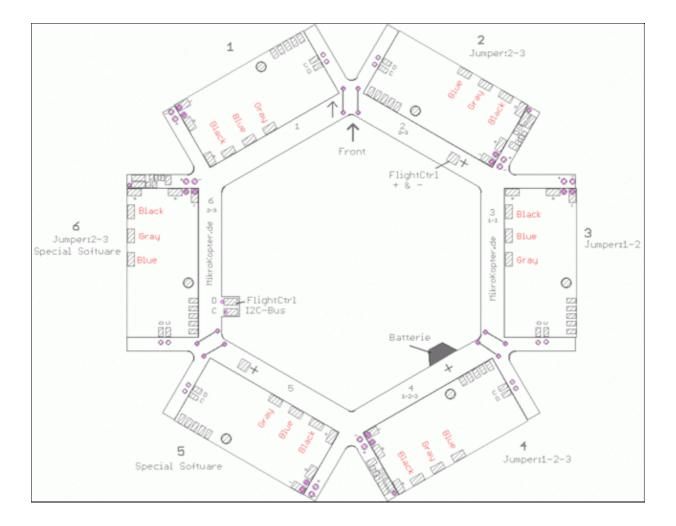
The BL-Ctrl's are arranged into the distribution board as shown.
