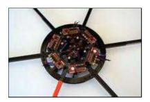
**ATTENTION**: The 10mm spacers on which the BL-Ctrl's are screwed tightly must be rotated so that the standoffs fully rest on the board of the respective BL-Ctrl. Please do not pinch the SMD capacitor C7!
