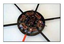
**ATTENTION**: The 10mm spacers on which the BL-Ctrl's are screwed tightly must be rotated so that the standoffs fully rest on the board of the respective BL-Ctrl. Please do not pinch the SMD capacitor C7!
