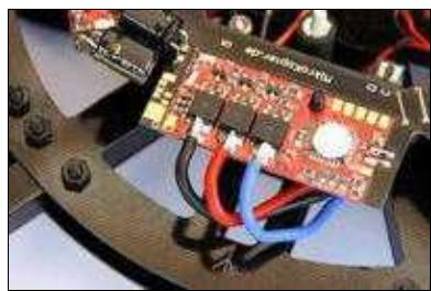
The cables of the engines for the BL-Ctrl 2,4,6 will be shortened accordingly, stripped, tinned well and soldered down from the "inside " to the respective BL-Ctrl. The connecting sequence doesn't matter right now. Maybe the sequence need to be switched for the start-up.
