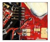
= Assembling of the FC = You can screw plastic nuts on the threads of the vibration damper so that the FC comes higher approx. 3mm. The  $\underline{\text{FlightCtrl}}$  will be mounted in the way that the small arrow points to the front. The FC will be tightened with four 15mm distance bolts.
