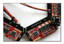
Battery cable: Silicon wire ca. 15cm / 2,5mm<sup>2</sup>
