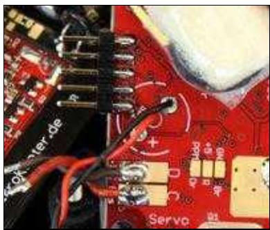
= Assembling of the FC = You can screw plastic nuts on the threads of the vibration damper so that the FC comes higher approx. 3mm. The [FlightCtrl](#) will be mounted in the way that the small arrow points to the front. The FC will be tightened with four 15mm distance bolts.
