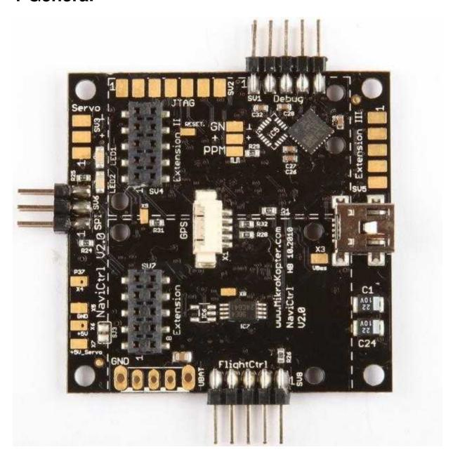
The <u>NaviCtrl</u> V2.0 with integrated compass is the follow of NaviCtrl V1.1 and expands with the **MKGPS** the ability of the MikroKopter.
