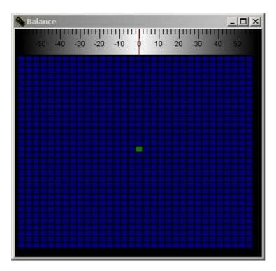
With the displayed center of gravity you can control while hovering if the Kopter has the center of gravity right in the middle or on a different spot.
