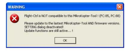
... then the <u>KopterTool</u> Version is not compatible to the software version on the <u>FlightCtrl</u> and/or <u>NaviCtrl</u>. Then you should update the <u>FlightCtrl</u> / <u>NaviCtrl</u> with the latest software version. (<u>Update</u>) (Alternatively, it could also be used an older version of <u>KopterTool</u>.)
