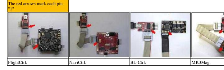
Are the boards, as shown in the pictures, individually connected, the jumper to supply power to the components should be closed on the MK-USB.
