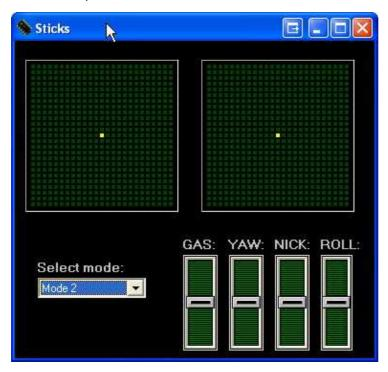
With this display you can check the function and the position of both control-sticks. Here you need to set in the display the used Mode on your transmitter (Mode 1-4).
