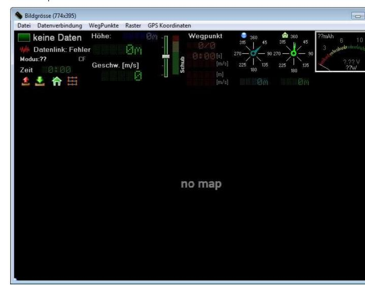
For the on-screen display (OSD) a data connection is required for the Kopter. This can be done via Bluetooth or Wi232.
