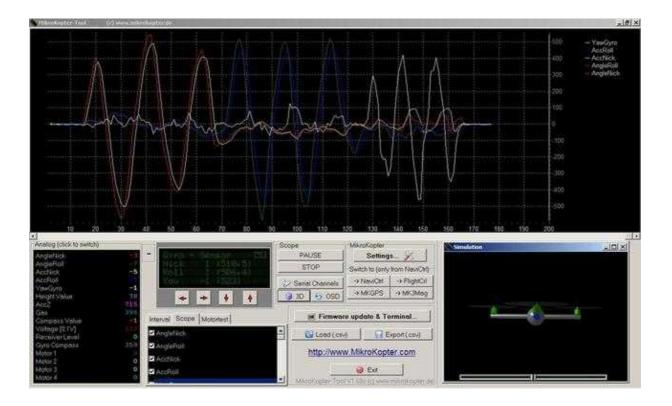
**Example:** FlightCtrl display for Nick, Roll, Yaw. To get the scope lines, the FlightCtrl must be inclined in the direction of it's corresponding talk: nick / turn!
