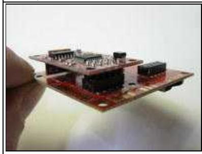
**⚠ Installation:** Use two plastic screws to fasten the MK3mag and avoid contact loss. In case of a bad contact, the GPS navigation could stop or the [MikroKopter](#) could fly into the wrong direction. Never use screws made of material that can become magnetic. When this screw becomes magnetic due to the engines, the compas function will get an offset, you will see this as a rotating Mikrokopter, directly after lift-off.
