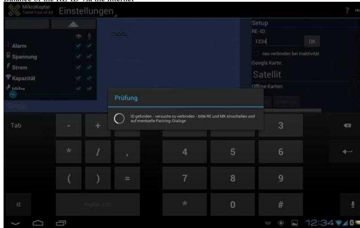
After a successful identification the tablet tool will bind with the RangeExtender - The blue LED on the RE flashes ...
