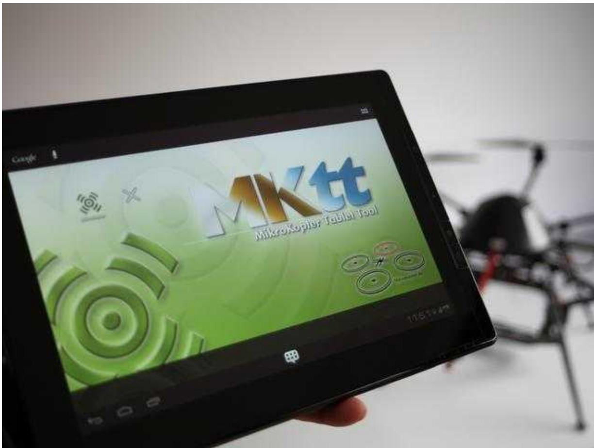
The MikroKopter-Tablet Tool (short: MK-TT) is an Android-APP which sets WayPoints and/or POI pretty easy into a map and can be transferred to the Kopter.
