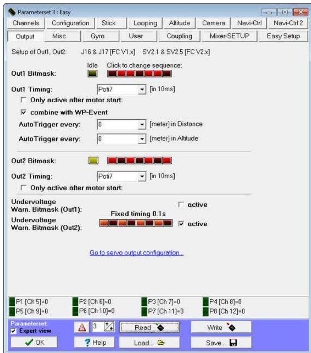
The two switching outputs of the FlightCtrl can be controlled and Set via the rider *Output*.
