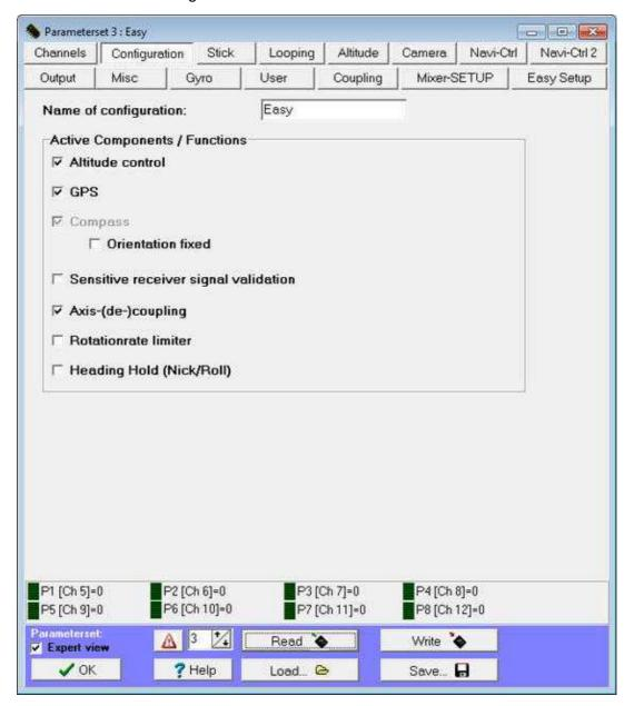
In a total of five sets of parameters different settings can be stored in the Kopter. These can be accessed through the sticks after turning on the Kopter and the initialization.
