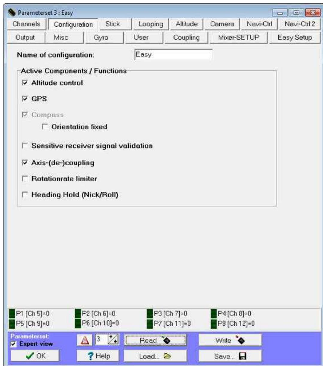
In a total of five sets of parameters different settings can be stored in the Kopter. These can be accessed through the sticks after turning on the Kopter and the initialization.
