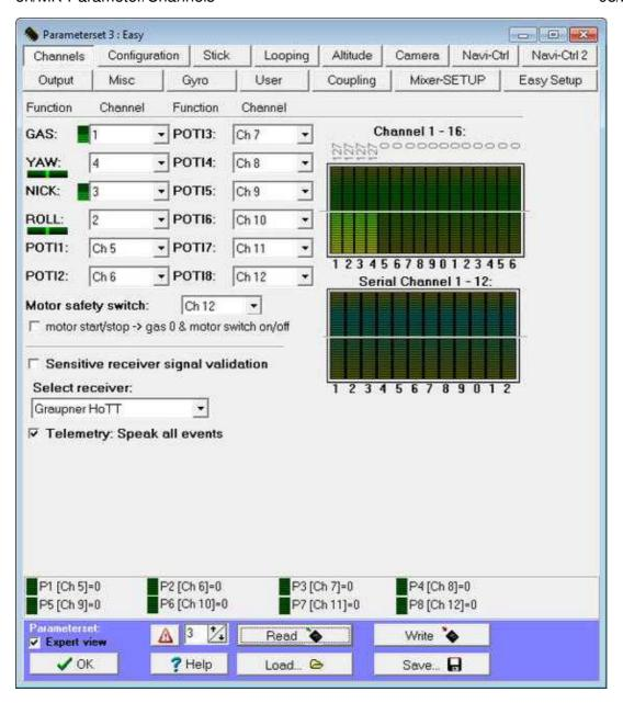
From software version V2.00 the FlightCtrl can handle up to 16 channels from the transmitter and up to 12 channels via a serial input.
