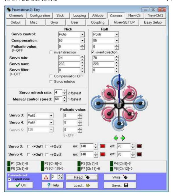
If a camera mount is used the function of the (pitch / roll) servos can be adjusted. These servos are connected to the connector SV2 => Servo1 (Nick) and SV3 => Servo2 (roll) of the FlightCtrl.
