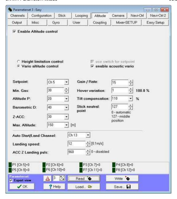
The altitude control on a !Mikrokopter is based on measuring the air pressure and z-axis accelerometer-/gps-values . A PID controller controls the overall thrust of all the rotors so that the measured air pressure (altitude) remains constant.
