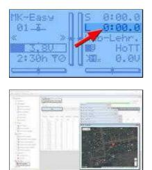
The telemetry data of the transmitter and also the position data of the copter are stored on a sd card in the transmitter.
