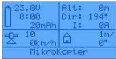
In the upper display of your transmitter you can see the MikroKopter-Telemetry. Here you can see:
