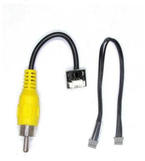
It is a control board incl. video output to operate cameras with a LANC interface (i.e. Sony cx730/cx760/cx570)
