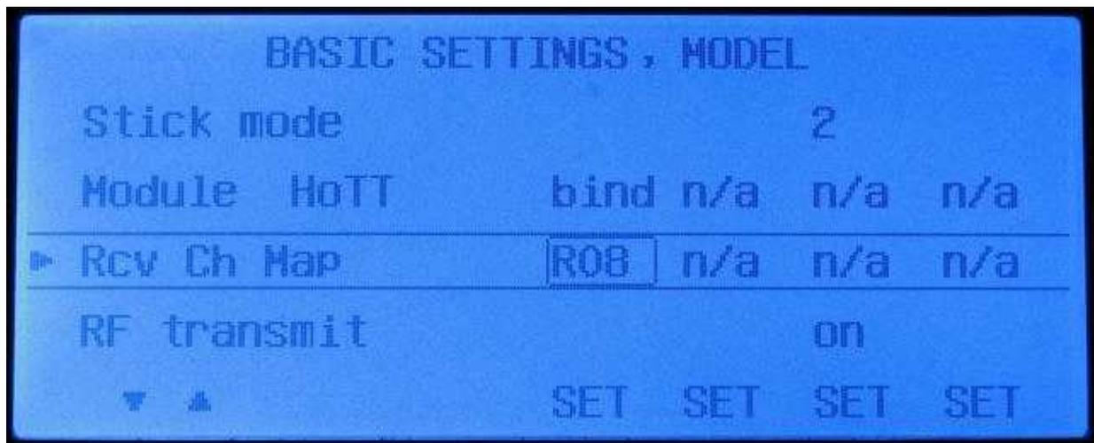
In the window which opens up choose the first servo output *Rx Output Ch 1* and set the *Rx Input Ch 1* to channel 11.
