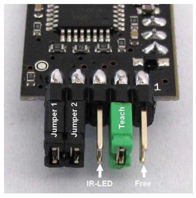
**① ATTENTION:** The plug of the IR-LED must be connected in that way that the red side points upwards (pointing to the IC).
