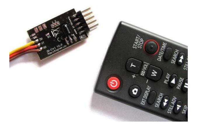
The red LED on the IR-Ctrl acknowledges the input with a unique flash - The green LED flashes again in second intervals.
