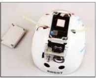
There is in the front a waterproofed <u>GoPrp</u> camera. And in the back the <u>FollowMe</u>-Transmitter with 9V batterie supply and a WI232 transmitter.
