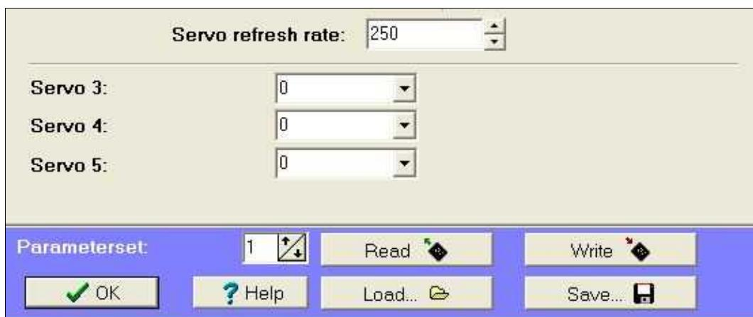
**⚠** Whether a channel will be controlled is dependent on the Refresh rate: If for example a 4 is entered here, then the maximum servo that will be controlled is Servo output 4
