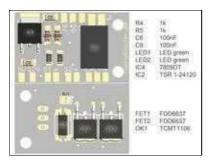
The board must still be equipped with the enclosed components. This requires a suitable soldering iron and basic knowledge in soldering.
