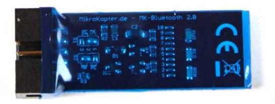
The enclosed ribbon cable will be connected with one side to the *MK-Bluetooth*. The other side is connected either to the <u>FlightCtrl</u> (EXT1) or when using the GPS-System to the <u>NaviCtrl</u> (Debug).
