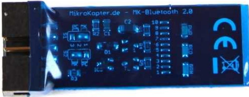
The enclosed ribbon cable will be connected with one side to the *MK-Bluetooth*. The other side is connected either to the [FlightCtrl](#) (EXT1) or when using the GPS-System to the [NaviCtrl](#) (Debug).
