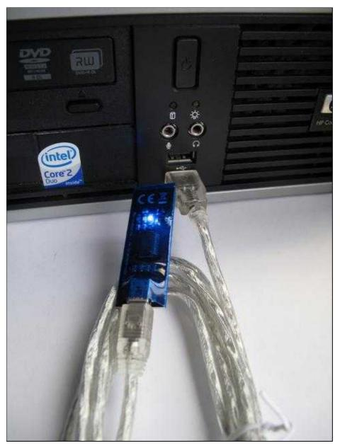
After connecting the *MK-Bluetooth-USB* the blue LED lights on, the module will be automatically detected and for the appropriate driver will be searched online as well as installed. This procedure can take a few minutes.
