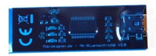
For the installation of the *MK-Bluetooth-USB* a VCP-Driver is necessary. This driver can be downloaded here: <u>VCP-Driver</u>
