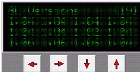
In case that there are different versions of BL-Firmware installed, the [KopterTool](#) (since V2.06e) shows the lowest version in the List:
