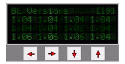
In case that there are different versions of BL-Firmware installed, the <u>KopterTool</u> (since V2.06e) shows the lowest version in the List:
