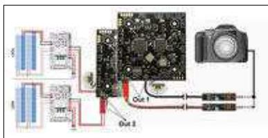
Anschlüsse FlightCtrl V3.0
