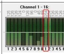
To use the Automatic during a Way point flight we have to change the settings for this channel on the transmitter. If you use e.g. a Graupner HoTT transmitter we find this setting under *Servo adjustment*: (in this example we use channel 11 to trigger the camera)
