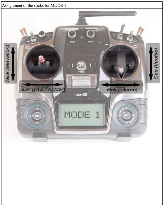
Description of the stick assignment for MODE 1 Calibration of the ACC Function (One time => necessary. The Kopter must stand Nick (elevation) straight.) Throttle up Description / Yaw right of the stick assignment / Nick middle / => Roll middle Roll (aileron) Gier (yaw / rudder) mx-20
