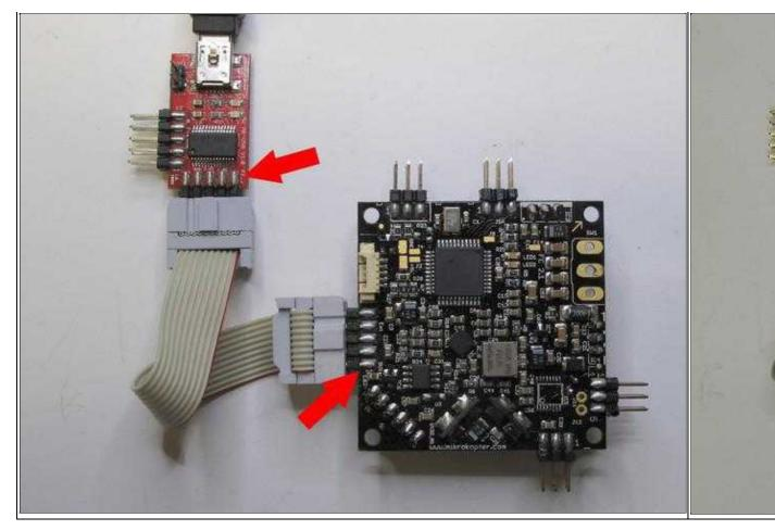
If the boards, as shown in the pictures, are individually connected, the voltage supply is supported by the MK-USB.
