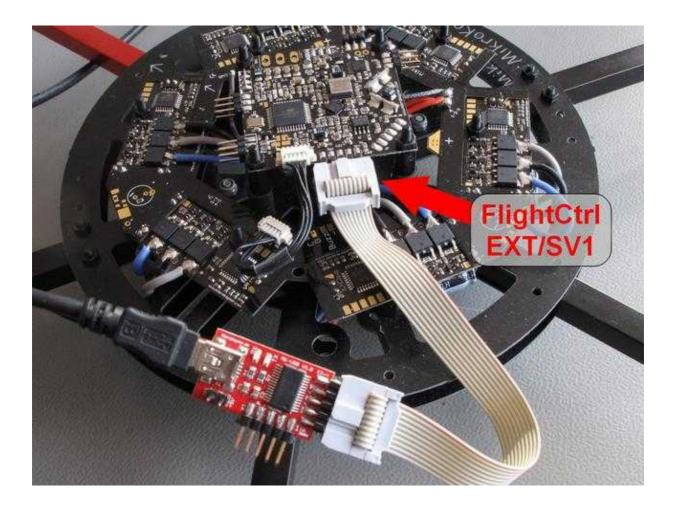
However, if the <u>MK-Tower</u> is used at the <u>MikroKopter</u> (FlightCtrl, NaviCtrl, MK3Mag, MK-GPS), the FlightCtrl and the NaviCtrl are connected over a 6-pin and one 10-pin cable. The <u>MK-USB</u> is plugged into the 10 pole interface "Debug" at the <u>NaviCtrl</u>.
