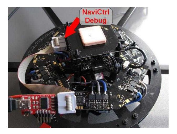
**The jumper on the MK-USB is still open.** To power the <u>MikroKopter</u>, please use the lipo or a power supply. A regulated power supply is particularly recommended for the first start of the <u>MikroKopter</u> to avoid damage to the Kopter
