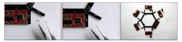
The silver wire will be stuck in the holes of the distribution-board and bent over. After that the ends of the wires will be soldered to the "C" and "D" connection pads of the BL-Ctrls.
