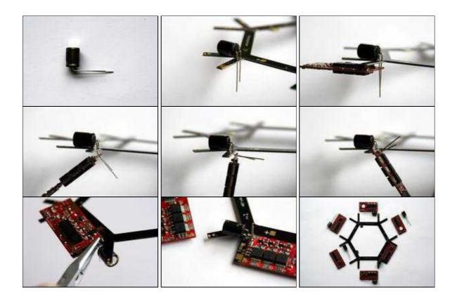
$\Delta$  You need to solder all Elkos carefully and with alot of heat otherwise you'll get pretty quick a cold solder-joint. The distribution-board is covered with 70µm copper so that more heat can be discharged to the sides.
