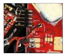
= Assembling of the FC = You can screw plastic nuts on the threads of the vibration damper so that the FC comes higher approx. 3mm. The <u>FlightCtrl</u> will be mounted in the way that the small arrow points to the front. The FC will be tightened with four 15mm distance bolts.
