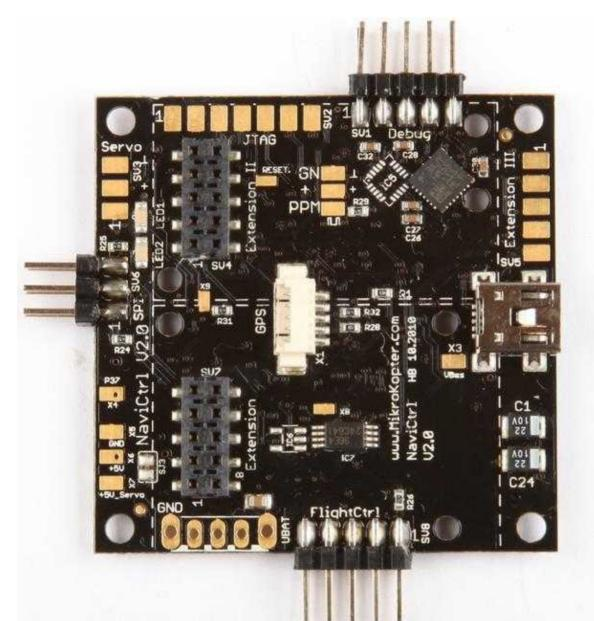
The **NaviCtrl V2.0** with integrated compass is the follow of NaviCtrl V1.1 and expands with the **MKGPS** the ability of the MikroKopter.
