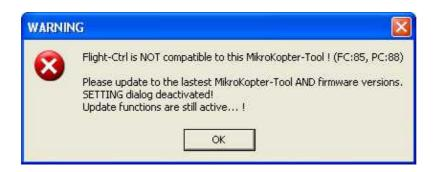
... then the <u>KopterTool</u> Version is not compatible to the software version on the <u>FlightCtrl</u> and/or <u>NaviCtrl</u>. Then you should update the <u>FlightCtrl</u> / <u>NaviCtrl</u> with the latest software version. (<u>Update</u>) (Alternatively, it could also be used an older version of <u>KopterTool</u>.)
