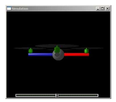
With this function you can display the function of the Gyros visually. The behavior of the 3D-Model is exact the same as the original.
