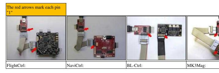
Are the boards, as shown in the pictures, individually connected, the jumper to supply power to the components should be closed on the MK-USB.
