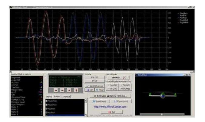
**Example:** <u>FlightCtrl</u> display for Nick, Roll, Yaw. To get the scope lines, the <u>FlightCtrl</u> must be inclined in the direction of it's corresponding talk: nick / turn!
