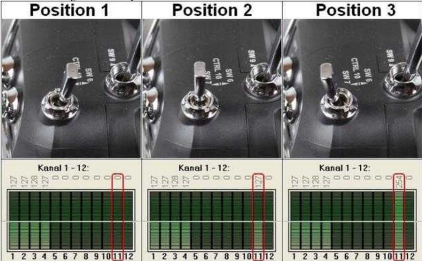
Channel 7 - assigned to a potentiometer or slider: Position 2 Position 3 Position 1 Kanal 1 - 12: Kanal 1 - 12: Kanal 1 - 12: 55850000000 558500B00000 228200000000 2 3 4 5 6 7 8 9 10 11 12 1 2 3 4 5 6 7 8 9 10 11 12 1 2 3 4 5 6 7 8 9 10 11 12 Position 1 Position 2 Position 3 Graupner/57 Graupner 57 Kanal 1 - 12: Kanal 1 - 12: Kanal 1 - 12: 0000 0000 00000 00元级成立 1 2 3 4 5 6 7 8 9 10 11 12 1 2 3 4 5 6 7 8 9 10 11 12 1 2 3 4 5 6 7 8 9 10 11 12
