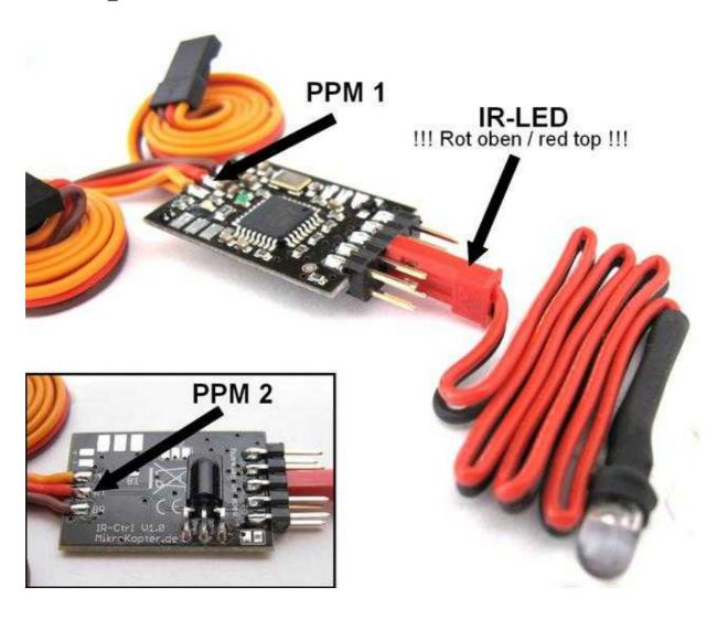
**① ATTENTION:** The plug of the LED must be connected in that way that the red side points upwards (pointing to the IC).
