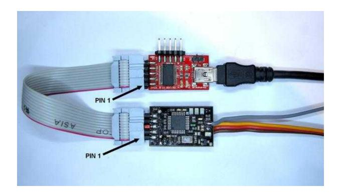
Via the <u>KopterTool</u> (from V1.78c) it is possible to refresh the LANC-Ctrl with new Updates or reset back into the delivery status.
