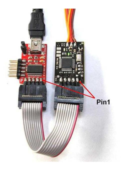
Via the <u>KopterTool</u> (from V1.78c) it is possible to refresh the IR-Ctrl with new Updates or reset back into the delivery status.
