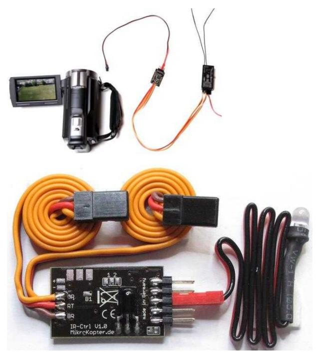
The **IR-Ctrl** is a control board to trigger cameras or video-cameras via infra-red.
