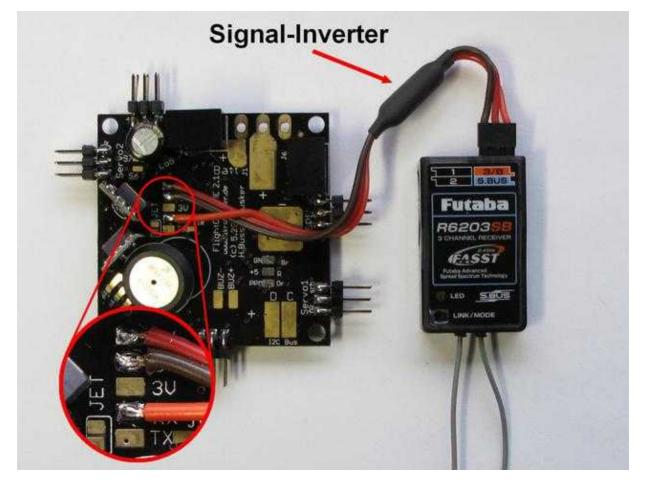
Since this version receiver from Futaba with the S.Bus will be also supported. Connected are those by a Signal-Inverter to the FlightCtrl.
