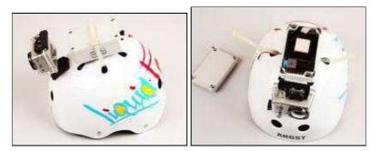
There is in the front a waterproofed <u>GoPrp</u> camera. And in the back the <u>FollowMe</u>-Transmitter with 9V batterie supply and a WI232 transmitter.
