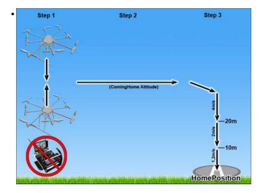
If the 60sec. are used up because of a to great distance or altitude to the homepoint, the pre-defined "EMERGENCY-Gas/Throttle" will be switched on automatically.
